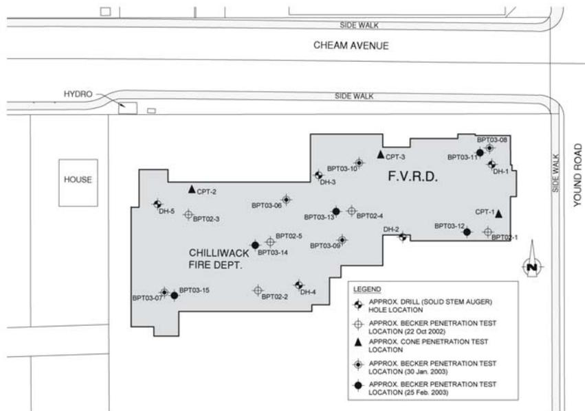
**Figure 2 Site plan with test hole locations.**
